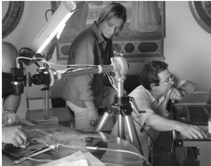
Figure 12. Localized vacuum consolidation of the paint film, monitored with the thermographic camera.
